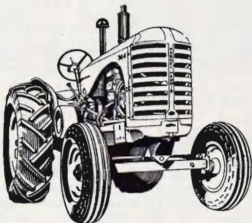
**RELIABILITY**— Produced with modern methods and equipment to the highest standards of British Engineering, the 744D is built throughout for a long working life. Its estimated horsepower, 29 drawbar, 36 belt, with maximum 39/42, gives ample power for general farm work. It has 6-cylinder smoothness, and all-day comfort for the driver on a "velvet-ride" hydraulic seat.
