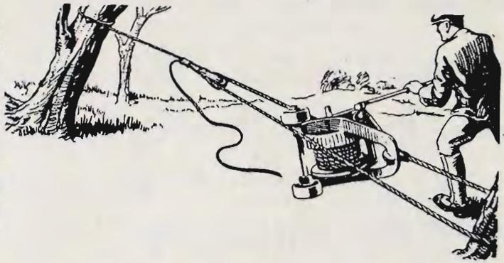
The machine is compact and sturdily built to deliver 260 times the power applied to the handle. It is quite portable and fitted with an automatic lowering gear, second speed, rope shortener, snatch block, etc. Ample cable to take an acre and a half from an anchor.
