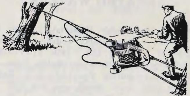
The machine is compact and sturdily built to deliver 260 times the power applied to the handle. It is quite portable and fitted with an automatic lowering gear, second speed, rope shortener, snatch block, etc. Ample cable to take an acre and a half from an anchor.
