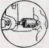
3. Spring tension engagement between cone and friction wheel, with one-point, readily accessible adjustment—for simpler, smoother shearing.
