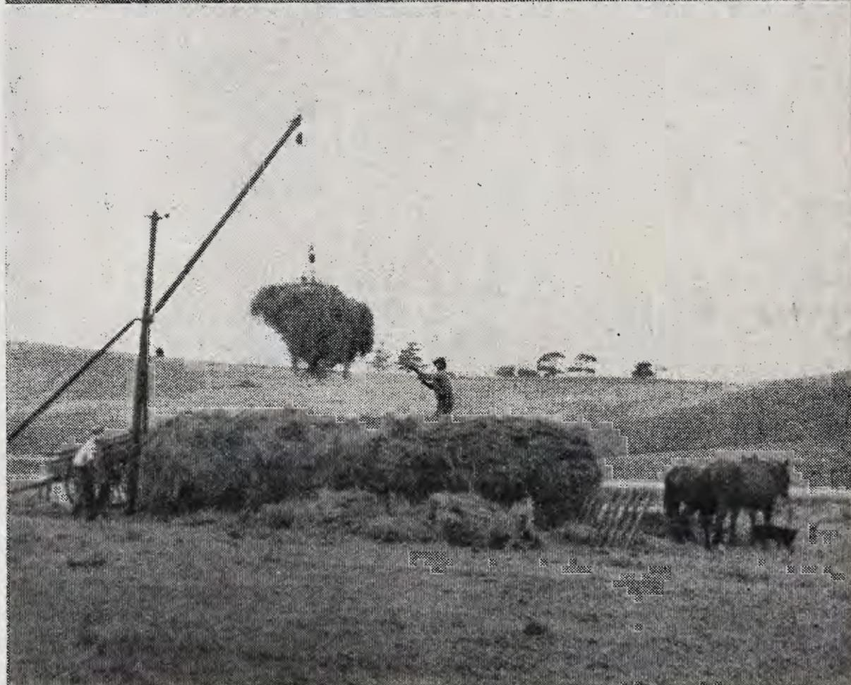
Above: Mechanical hay loader adapted for handling green material for silage.
