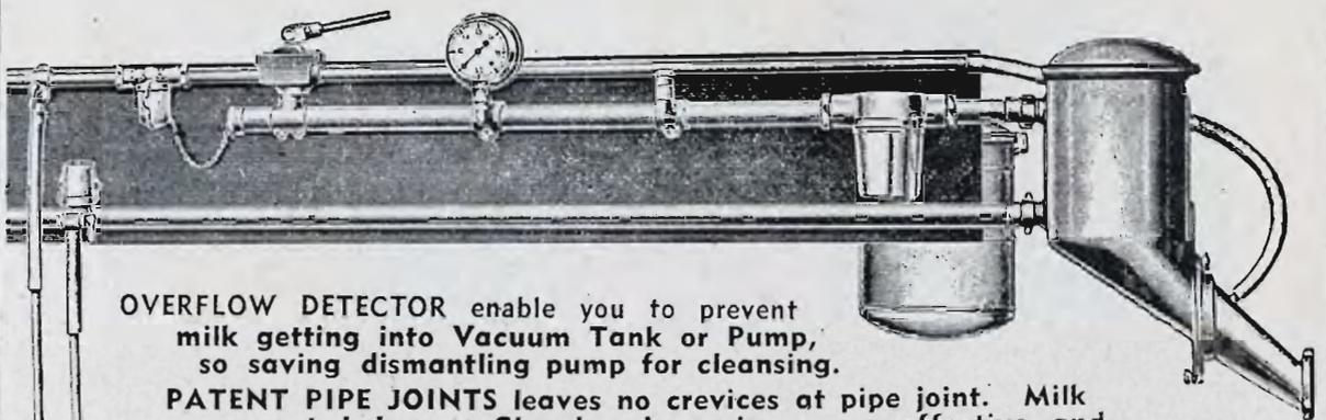
**OVERFLOW DETECTOR** enable you to prevent milk getting into Vacuum Tank or Pump, so saving dismantling pump for cleansing.
